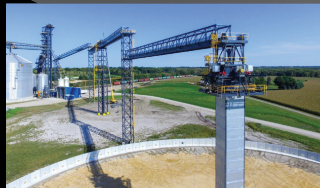
Complete temporary storage systems consisting of center air tower, conveyor trusses, support towers, Material handling, tarp and aeration tubing
